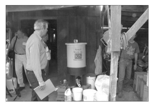
A 28-gallon KIS brewer in action at a local farm near Corvallis, Oregon. Excellent tea with high biomass of bacteria, fungi and protozoa is consistently produced with this machine. Data for this machine can be found at <www.simplici-tea.com>.
